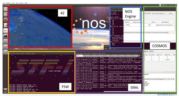
Figure 8 - NOS3 Running - Server, Sumulators, 42, Flight Software, COSMOS
